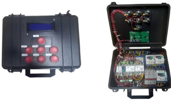
Figure 7. Display of control components: ESP32 module, electrical safety, and current distribution system.
