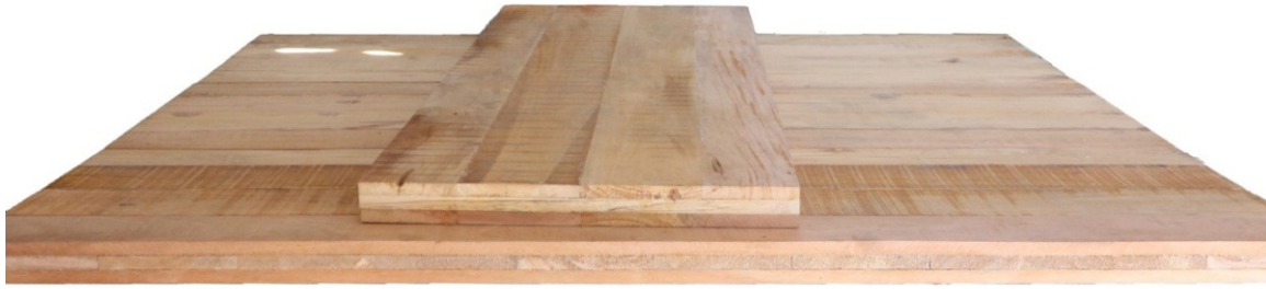
Figure 3. Cross-laminated timber (CLT) of mahogany-sengon-mahogany (Widyorini et al. 2023)
