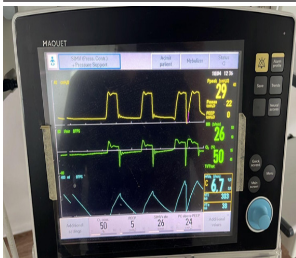
Figure 1. Ventilator screen display while the patient was intubated with a size 4 cuffed endotracheal tube (pediatric ventilation mode, elevated peak airway pressure, and low tidal volume
