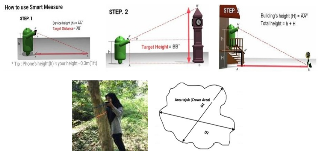
Figure 2. Measurement of physical factors of Syzygium trees. (a) Illustration of tree height measurement using smartmeasure . (b) Measurement of tree diameter. (c) Illustration of crown area measurement (Hematang et al. 2021).
