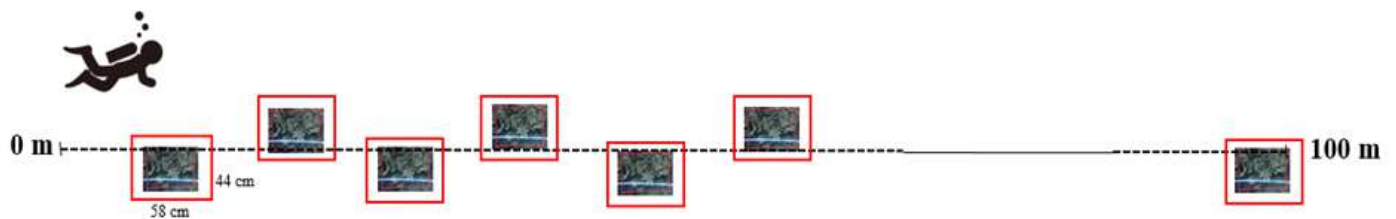
Figure 2. Placement frame which is marked with a red box with dimensions of 44 cm x 58 cm on roll meter 100 m long is used for Underwater Photo Transect (UPT) in coral reef ecosystems and Photos of the transects from the right and left sides.
